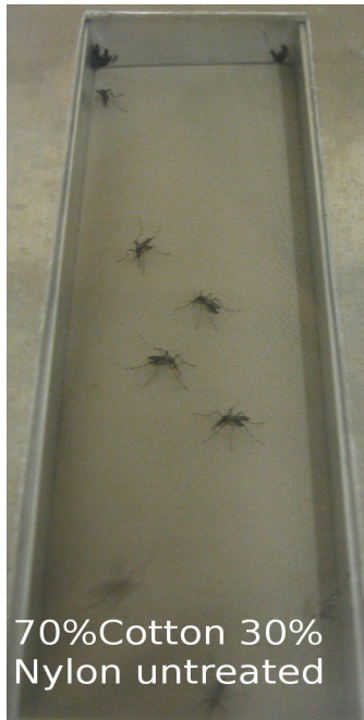
Figures 10 & 11 : Tests of untreated and treated 70% Co 30% Ny samples on volunteer A
