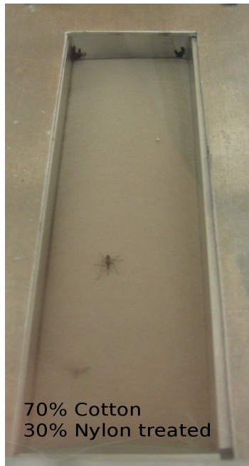
Figures 10 & 11 : Tests of untreated and treated 70% Co 30% Ny samples on volunteer A
