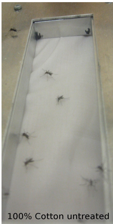
Figures 12 & 13 : Tests of untreated and treated 100% Cotton samples on volunteer B
