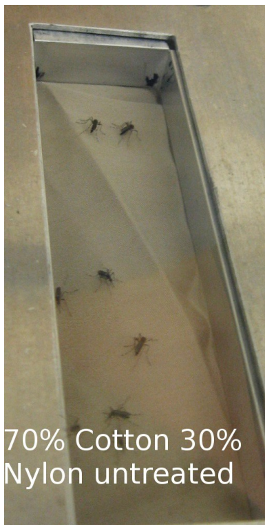
Figures 20 & 21 : Tests of untreated and treated 70% Co 30% Ny samples on volunteer B
